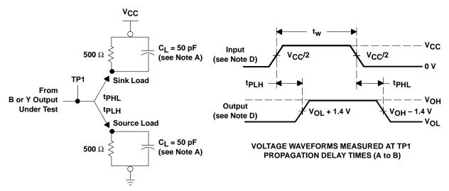
A-TO-B LOAD OR A-TO-Y LOAD (Totem Pole)
